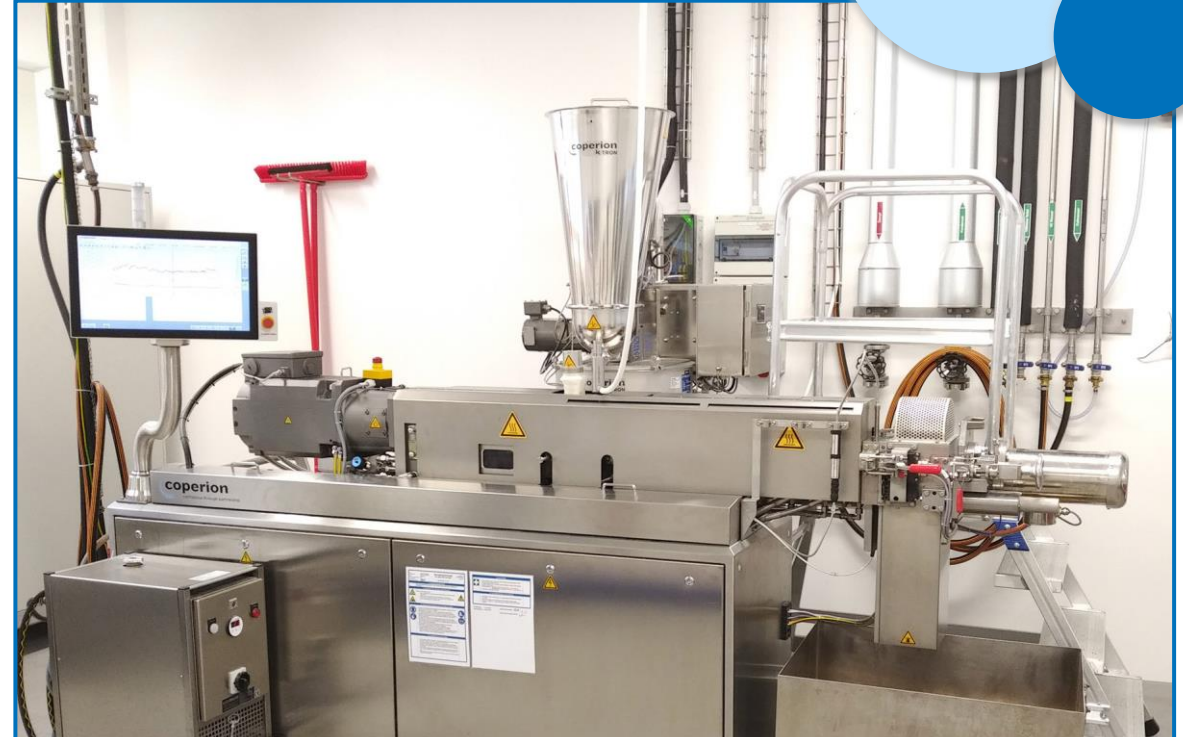
Production of textured proteins in the pilot extruder for meat substitute products in Offstein/Germany
